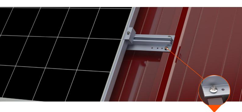
Installing the Quick RAIL mounting structure produces no swarf thanks to our special screws that create their own extended thread. Why is this important? With stepping on swarf during installation, micro-cracks occur in your roof structure. The damage is not visible right away, but certainly with time it has a major negative effect on the roofing properties.
